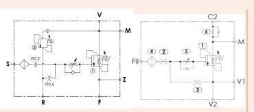
Maximum operating pressure:500 barRated flow:up 80 l/minManifold material:Steel
