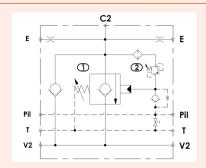
Maximum operating pressure: 420 bar Rated flow: up 400 l/min Manifold material: Cast Iron Surface treatment: Zinc Nickel plating
